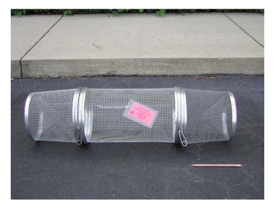
Figure N: Standard Eel Pot that was Used Throughout Sampling
